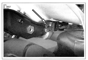
Figure 4-11. Purge Solenoid (mudflap removed)
