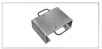
Part No. HD-45317 Engine Assembly Support Fixture
