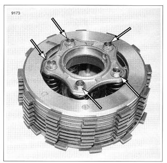
Figure 3-88. Lifter Plate Fasteners
