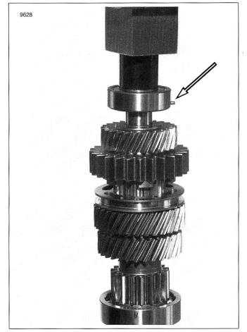
Figure 7-38. 2nd Gear Bearing Alignment Pin
