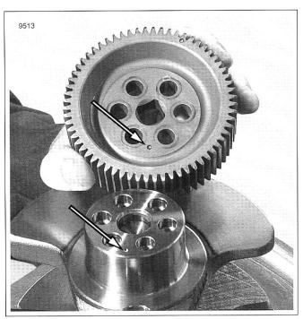
Figure 3-209. Primary Gear Timing Marks
