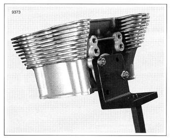
Figure 3-58. Cylinder Head Holder
