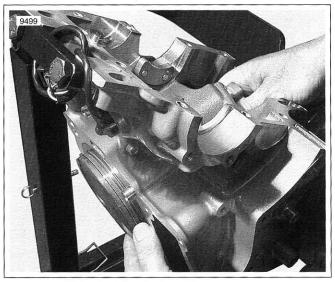
Figure 3-200. Remove Pistons
