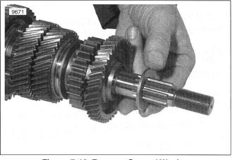
Figure 7-13. Remove Ground Washer
