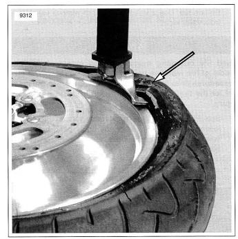
Figure 2-81. Tire Machine Pulling Bead Off Rim
