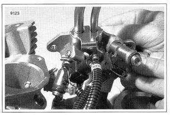
Figure 3-14. Fuel Rail with Injectors
