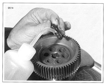
Figure 3-210. Installing Primary Gear
