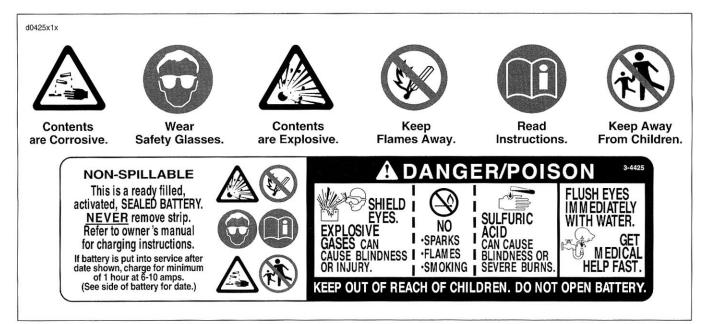
Figure 1-19. Battery Warning Label
