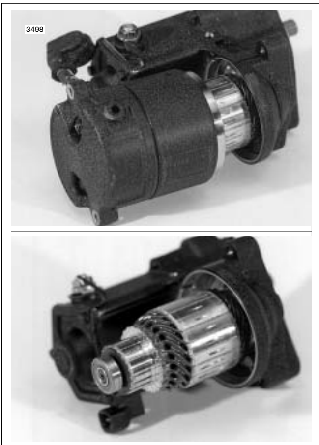
Figure 5-6. Remove Field Coil and Cap
