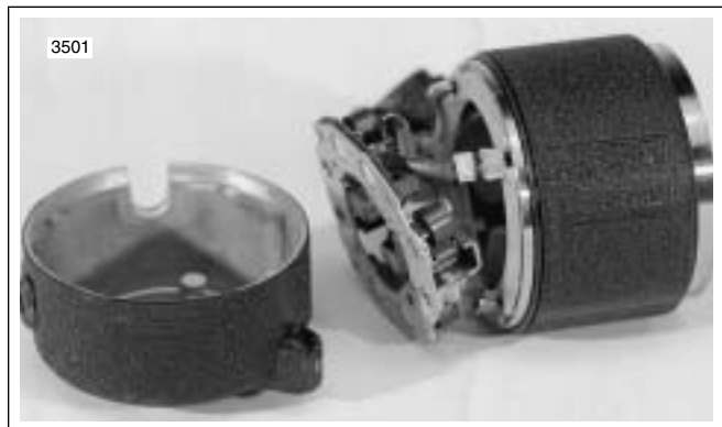
Figure 5-8. Remove End Cap
