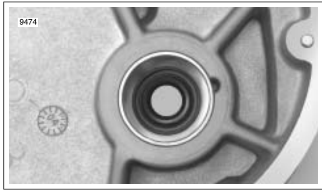
Figure 6-26. Install Jackshaft Lip Seal with Open Side of Seal Carrier on the Clutch Side
