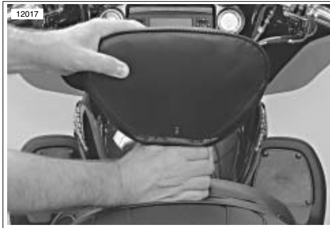
Figure 2-46. Removing Backrest
