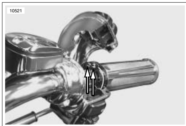
Figure 2-28. Throttle and Idle Cable Ferrules
