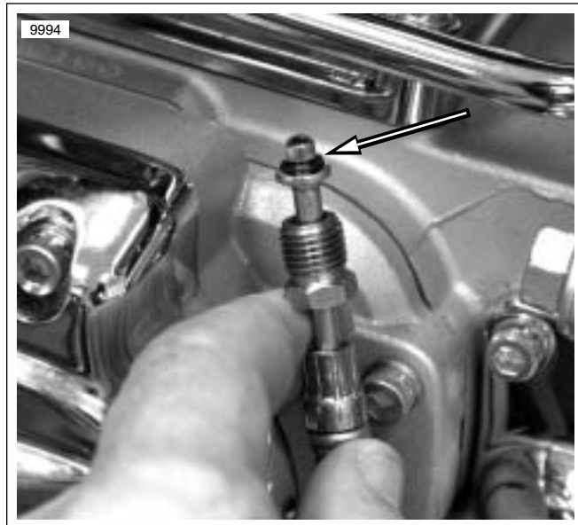
Figure 2-36. Clutch Fluid Line O-ring
