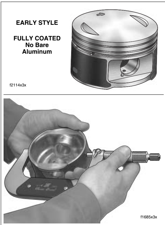
Figure 3-87. Measure Early Style Piston for Running Clearance
