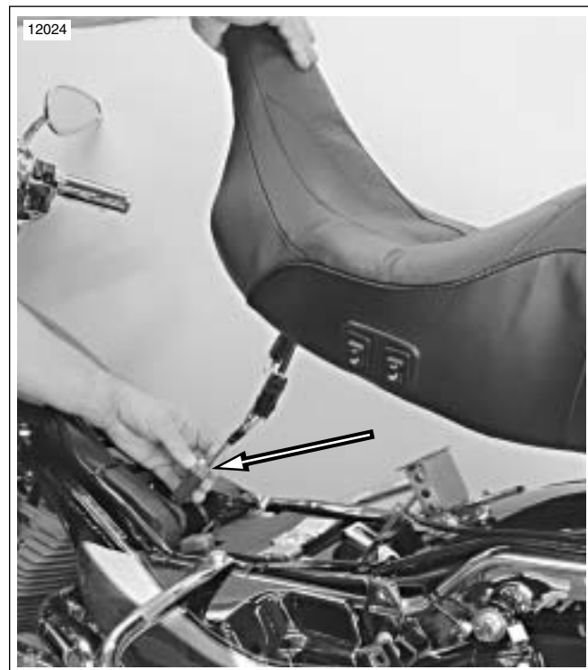
Figure 2-43. Seat Heater Connector [191]
