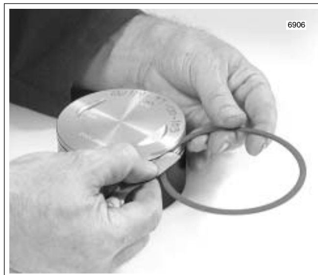
Figure 3-86. Measure Piston Ring Side Clearance
