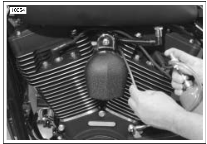
Figure 4-14. Checking for Leaks
