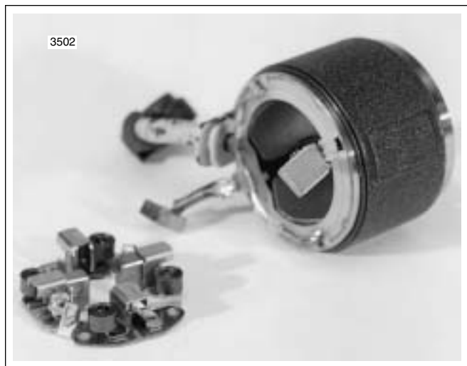
Figure 5-9. Remove Brush Holder
