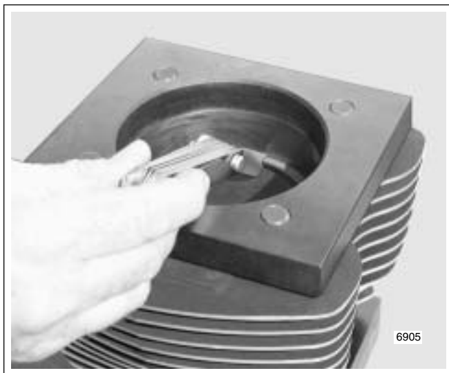
Figure 3-89. Measure Ring End Gap
