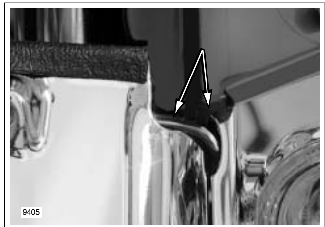
Figure 8-63. Route Conduit Thru Mounting Bracket and Chrome Skirt Reliefs (FLHX)
