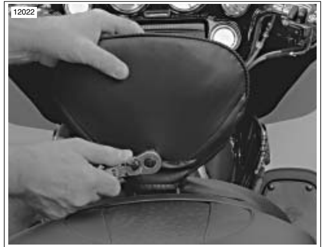
Figure 2-48. Adjusting Backrest Tilt Angle
