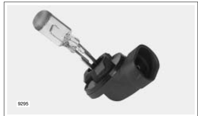
Figure 8-34. Auxiliary Lamp Bulb/Pin Housing
