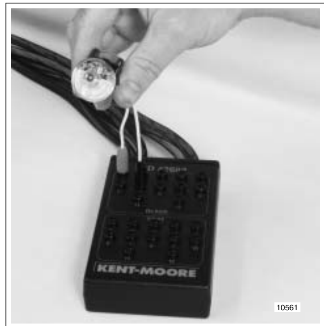
Figure 4-16. Ignition Coil Circuit Test
