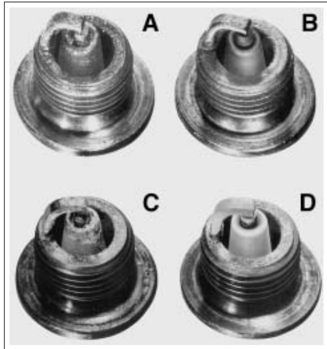
Figure 8-10. Types of Plug Base Deposits
