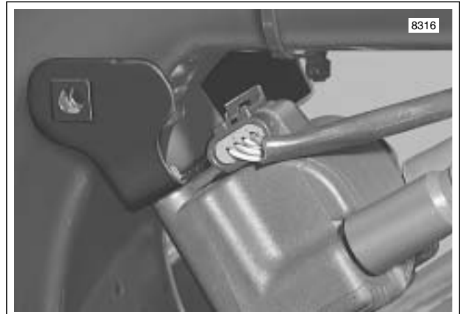
Figure 8-8. Remove Ignition Coil Bracket From Vehicle
