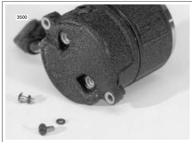
Figure 5-7. Remove End Cap Screws and O-Rings
