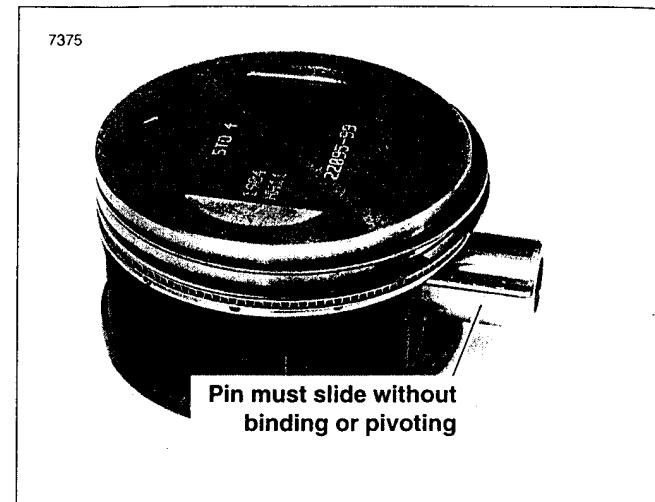
Figure 3-114. Piston Pin Clearance
